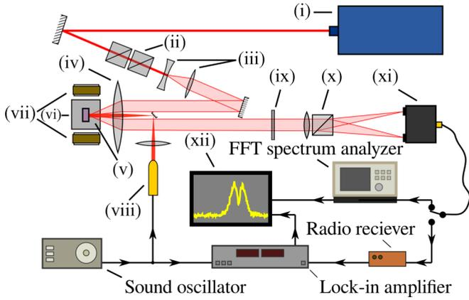
FIG. 1. (Color online) Schematic of the experimental setup.
