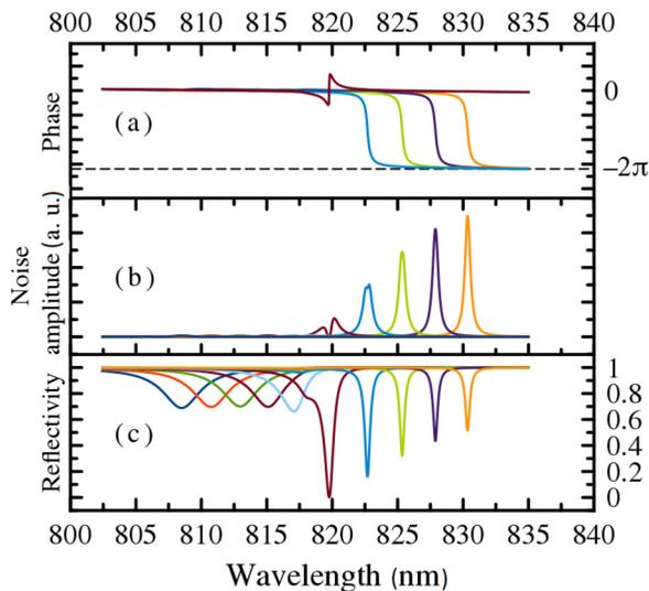
FIG. 5. (Color online) The calculated (a) phase of the reflection coefficient, (b) OSN spectra, and (c) reflectivity spectra of the asymmetric microcavity with QW at different spectral position of the photon mode. The QW permittivity was taken in the form  $\varepsilon(\omega) = \varepsilon_b + C \ln(\omega_0 - \omega + i\gamma)$ , with spectral position  $\omega_0$  corresponding to the center of the shown spectral range.
