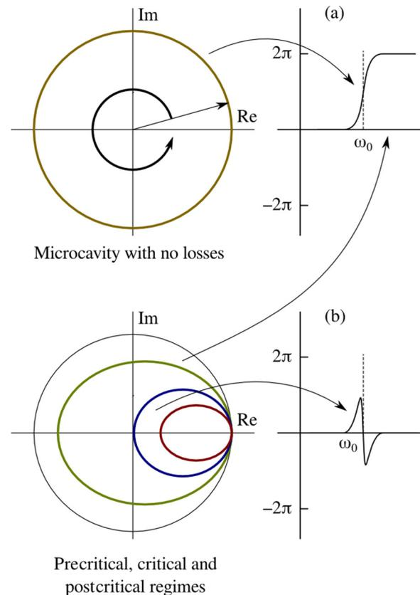
FIG. 3. (Color online) Dynamics of the complex reflectivity vector of the asymmetric cavity upon passing through the resonance. (a) Ideal (ultimate) asymmetric cavity; (b) asymmetric cavity at different absorption in the intermirror gap. The right plots show phase of the cavity reflection coefficient in the precritical and postcritical regime.
