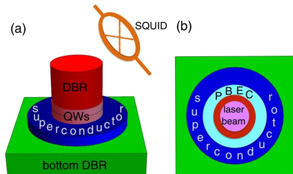
FIG. 1. The diagram of a structure suitable for observation of the interplay of phonon- and exciton (bogolon)-induced superconductivity. A superconducting ring is deposited around pillar semiconductor microcavity. DBRs denote distributed Bragg reflectors. The condensate of polaritons is excited by a laser (a). View from the top (b).
